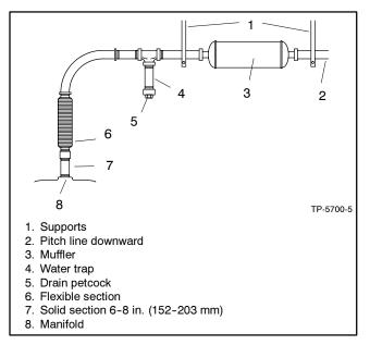
Figure 5-1 Exhaust System, End Inlet Silencer
